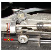
With the emergency cable released the clearance X indicated above must be adjusted to 1.0 to 2.0 mm.
