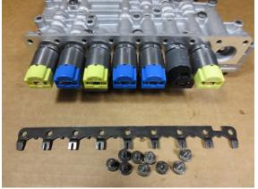
Remove the solenoid bracket screws and bracket.
