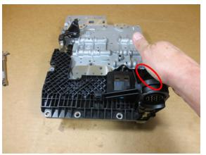
Insert and hand tighten the seven screws that hold the black plastic housing in place. Double check that the manual valve is properly engaged into the position slider switch and that the valve is moving freely.
