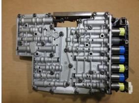
Stand the mechatronic up on its side as shown and remove the 7 screws indicated by the red circles.
