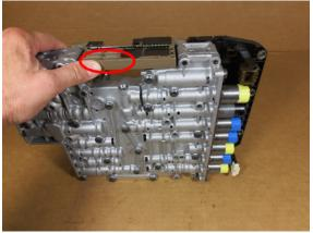
Separate the black plastic housing from the aluminum portion of the mechatronic. Place the housing in front of you as shown.
