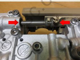
Torque the seven mounting screws to 5 Nm. You now have successfully replaced the mechatronic solenoids and are ready to reinstall the mechatronic.
