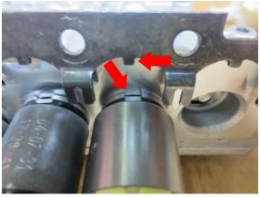
Reinstall the solenoid bracket and install all screws by hand, torque the screws to 5 Nm. Turn the mechatronic housing and place it in front of you as shown.
