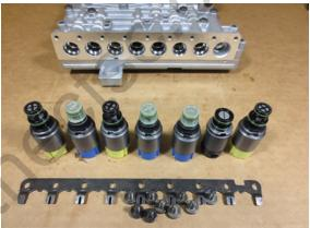
Unpack the new solenoids, follow the color sequence of the old solenoids and push the new ones into place. You might have to slightly wiggle the solenoid to be able to push it into place. Install the solenoids with the notch facing up a s shown. The notch in the solenoid needs to line up with the tab of the solenoid bracket. **NOTE:** Depending on the build date of your mechatronic, you might have yellow and green solenoids. The green solenoids are replaced by the blue ones.
