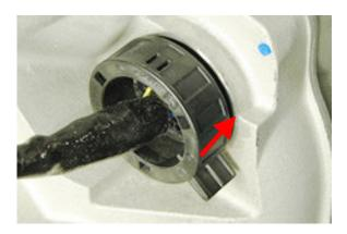
The Mechatronic (electronic valve body) located within the transmission is a electrostatic sensitive device, avoid touching any electrical pins to prevent ESD (electrostatic discharge) damage.
