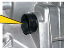
3. Pull the sealing sleeve locking mechanism to the unlocked position.
