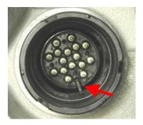
6. Push the sealing sleeve locking mechanism up into the locked position. Do not force the locking mechanism, if hard to lock, check that the sleeve is pushed in far enough with gap x smaller 3.0mm.
