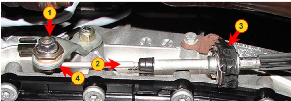
Always check the shifter cable bracket **3** to make sure it was not bent during transmission removal.
