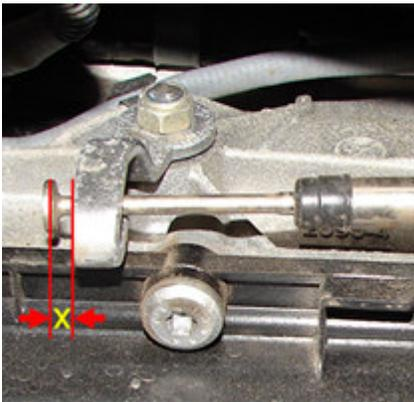
With the emergency cable released the clearance X indicated above must be adjusted to 1.0 to 2.0 mm.
