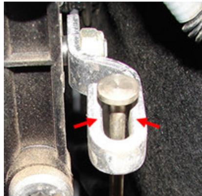
The cable should not touch the lever at any time, even if the lever is moved back and forth. If the cable does come in contact then check for a bent lever or a bent cable bracket.
