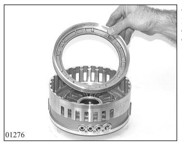
Turn cylinder CD by 180°. Pull 2 O-ring seals 75.040 and 75.050 onto piston C 75.030 and press it into the cylinder.
