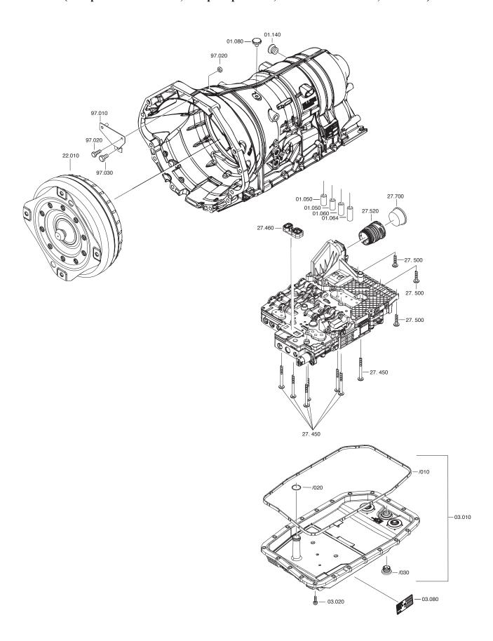
Turn the casing by 90°. Drive 4 sealing sleeves (2x 01.050, 01.060, 01.064) between the transmission casing and cylinder CD with a suitable tool.
