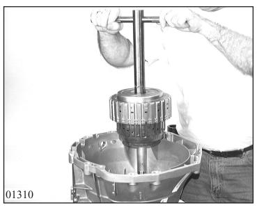
Place assembly tool 5x46 002 563 over the innput shaft and lock with pin. Align disks of clutch B, insert turret and turning it in both directions until the disks engage fully in disk carrier B.
