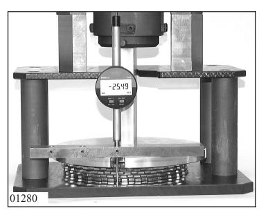
Determine thickness  $M_C$  of brake C clutch pack according to Chapter 1.4.0 Measuring clutch pack.
