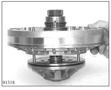
Screw locating pins 5x46 001 007 into pump. Mount complete pump over stator shaft, remove locating pins and tighten down with 11 machine screws 10.050.
