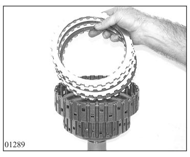
Determine thickness  $\mathbf{M}_{\mathbf{B}}$  of clutch B clutch pack according to Chapter 1.4.0 Measuring clutch pack.
