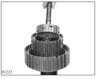
Lift off intermediate shaft with internal disk carrier E. Lever out axial needle roller bearing.
