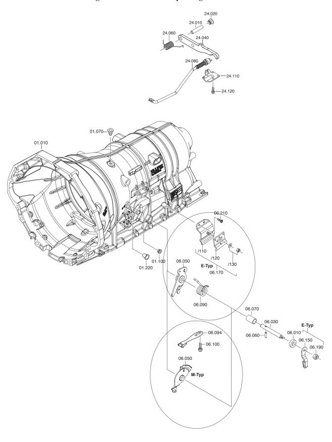
Drive breather 01.070 into transmission casing 01.010 with a plastic-faced hammer.
