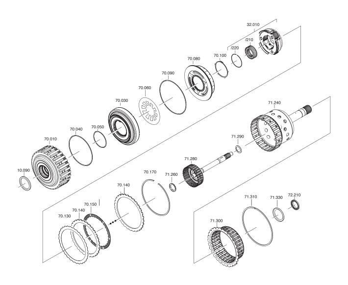
Pull 2 O-ring seals 70.040 + 70.050 onto piston A 70.030. Press piston A into cylinder A 70.010.
