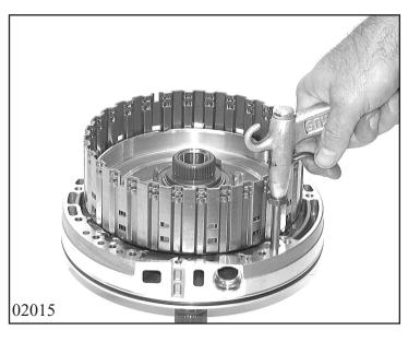
Place cylinder A on top of the oil supply and press out piston with compressed air. Pull 2 O-ring seals off piston A. Remove cylinder A from oil supply
