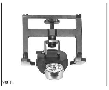
Using the knurled screw, turn adjusting device 5p01 001 458 to the upper limit.
