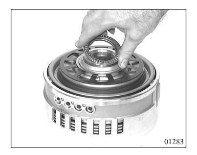
Insert complete clutch pack D into housing, starting with final disk 73.260, then insert lined disk 73.250 and external disk 73.240 alternately.
