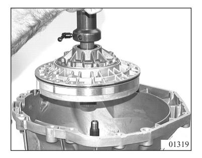
Tighten down the oil supply with 14 Torx screws and new Usit rings as follows:
