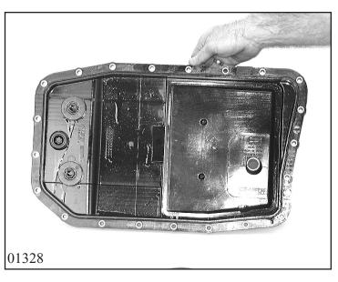
Pull new O-ring seal 03.010/020 onto stub pipe of oil filter 03.010. Press new seal 03.010/010 into oil pan.
