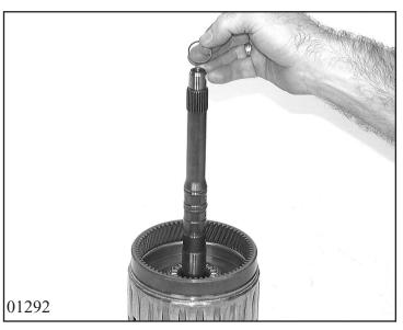
Pull 3 new rectangular-section rings 71.190 onto cylinder E 71.010 with input shaft.
