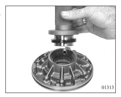
Pull on new O-ring seal 10.020. Lubricate the pump wheel and internal ring gear lightly before assembly. Then assemble the pump in such a way that one marking is visible both on the pump wheel and the internal ring gear.
