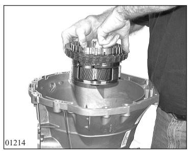
Take out the angle plate and sun gear. Remove planet carrier with complete clutch pack D.
