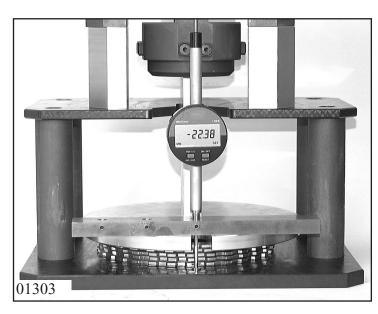
Determine thickness  $M_A$  of clutch A clutch pack according to Chapter 1.4.0 Measuring clutch pack.
