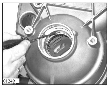
Remove the snap ring with pliers. If necessary, heat the casing around the needle roller bearing with a fan heater to 70° C. Turn housing with output side down and remove the needle roller bearing from the transmission casing.
