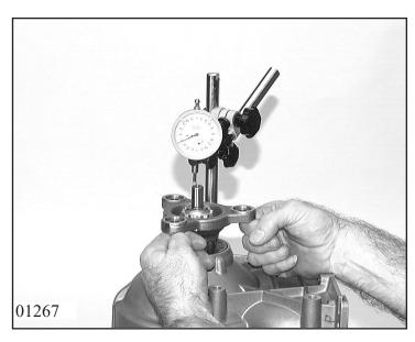
Pull on flange and read off value **A**. Select a thinner or thicker disk if value A is outside tolerance C.
