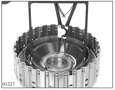
Press down cup spring in the mandrel press with assembly bracket 5x46 002 566 and remove snap ring with suitable pliers. Take out planet carrier and cup spring.
