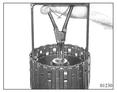
Cover one of the two oil guide bores and press out piston E with compressed air. Pull off the two O-ring seals.
