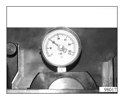
Then place measuring bar 5p01 060 330 on the measuring plate, put the dial gauge's measuring base in the measuring plate's groove on the top disc of the set, and set the dial gauge to 0.
