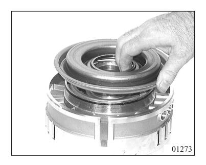
Pull 1 O-ring seal 73.070 onto baffle plate D 73.060 and press it into piston D. Press the air baffle plate down and secure with split retaining ring 73.100+73.110.
