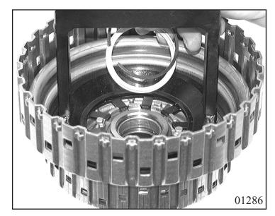
Insert complete clutch pack B, starting with spring disk 72.130. Then insert outer disk 72.140 and lined disk 72.150 alternately.
