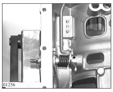
Insert parking or detent disk with connecting rod into transmission casing and push selector shaft 06.030 in through sleeve 06.070 and detent disk.
