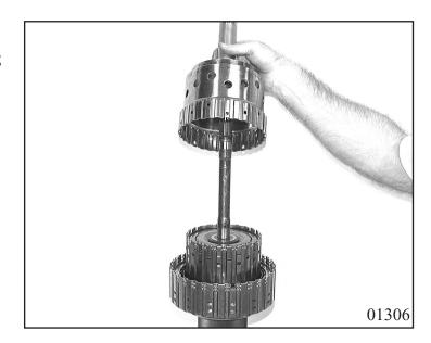
Insert inner disk carrier B 71.300 into cylinder A and secure with snap ring 71.310.
