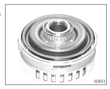
Insert cup spring 73.120. Press cup spring down in the mandrel press with assembly bracket 5x46 000 221 and secure with split retaining ring 73.130.
