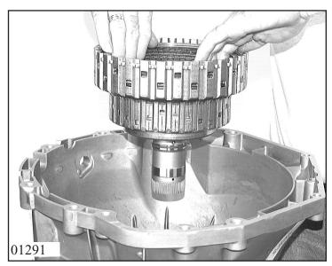
Insert angular disk 75.200 and also complete clutch B into transmission housing.
