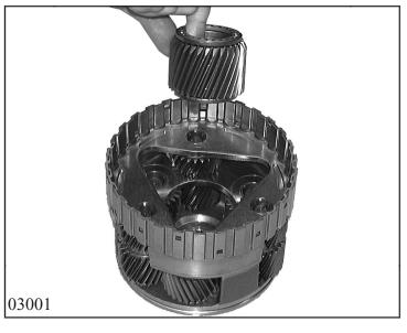
Remove thrust plates and sun gears 2 + 3 from planet carrier.
