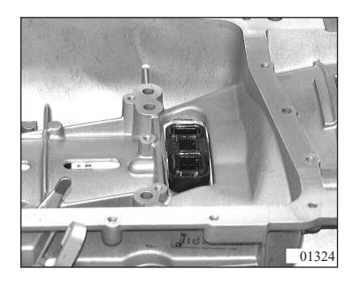
Check all clutches / brakes for proper function by supplying compressed air to the marked bores (see picture alongside)
