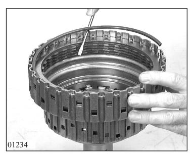
Turn cylinder by 180°, take out clutch B snap ring and take out the complete clutch pack.
