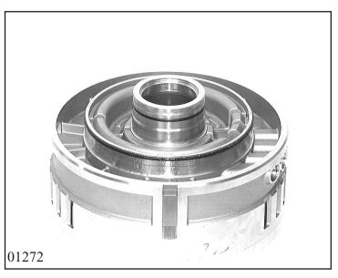
Drive 2 shaft keys 75.010/140 in centrally at cylinder CD 75.010, using a plastic hammer.
