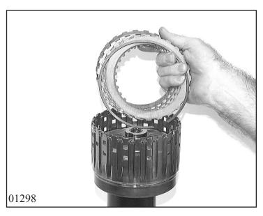
Insert complete clutch pack E. Start with spring disk 71.140, then insert outer disk 71.150 and lined disk 71.160 alternately. Insert final disk 71.150 and secure with snap ring 71.180.
