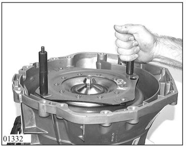
Turn transmission by 90° and move converter back and forward until the pump drive pins engage.
