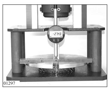
Determine thickness  $M_E$  of clutch E clutch pack according to Chapter 1.4.0 Measuring clutch pack.
