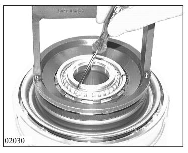
Turn the cylinder around and press down cup spring D in the mandrel press with assembly bracket 5x46 000 221; take out split retaining ring, stop ring and remove cup spring.
