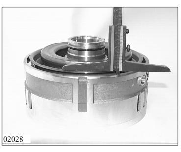
Measure down from piston to cylinder support area CD and read off dimension  $\ ^{\ }\square ^{\ }M_{DB}.$
