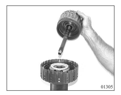
Align disks of clutches A and E and insert intermediate shaft 71.280, turning it while doing so.
