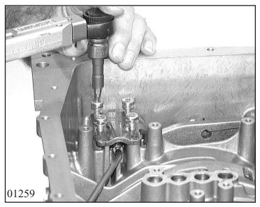
Press down ratchet and fasten guide plate 24.110 with 4 Torx screws 24.120.
