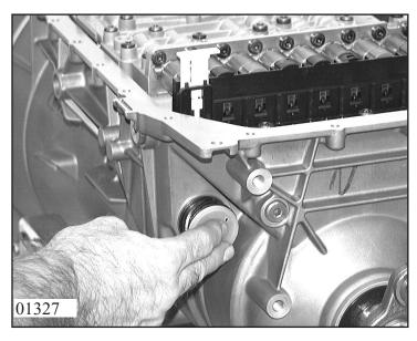
Press in new socket 27.520 D with mechatronics screw plug 27.700 attached D and secure with retaining clip. J
