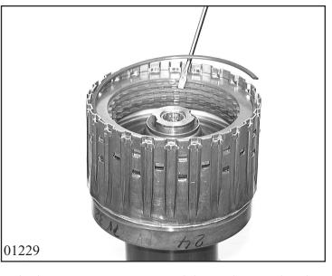
Pull out clutch E snap ring and withdraw complete clutch pack of clutch E.
