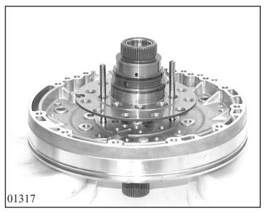
Put the intermediate and centering plates on a supporting fixture and heat up with a hot-air blower to approx. 70 °C.
