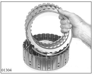
Insert complete clutch pack A. Start with spring disk 70.130, then insert outer disk 70.140 and lined disk 70.150 alternately. Secure the top outer disk 70.140 with snap ring 70.170.
