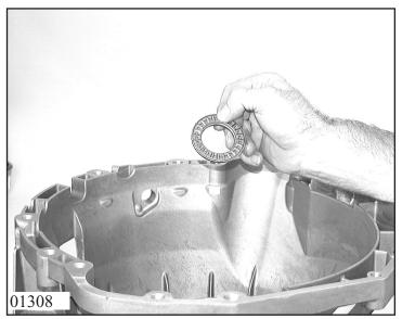
Place axial needle roller cage 72.210 on the hub of cylinder B. Note correct installed position of bearing, see picture alongside.
