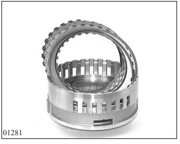
Insert complete clutch pack C into cylinder CD, starting with spring disk 75.100.
