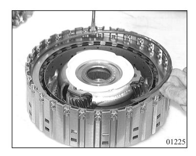
Lever snap ring out of planet carrier and take planet carrier out of cylinder A. Withdraw snap ring and sun gear from planet carrier and lever out axial needle roller bearing cage.
