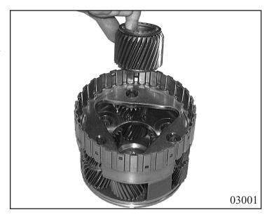
Turn transmission with converter bell upwards.
