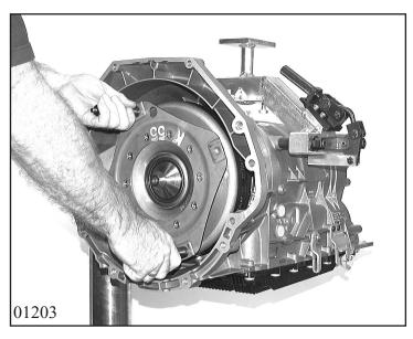
Remove converter bracket and take out converter
