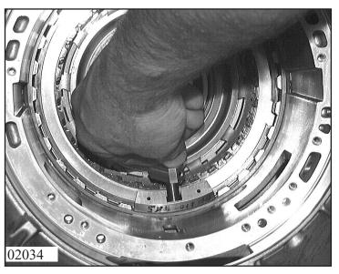
Secure with snap ring 73.210. Use driving-in tool 5x46 001 930 to drive the snap ring into the housing groove all round.
