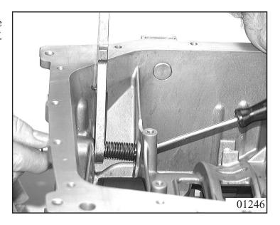
Remove the shaft sealing ring from the transmission casing with a suitable lever. Remove the snap ring with pliers.
