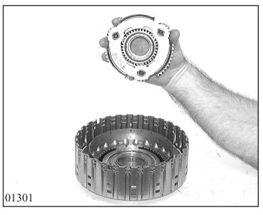
Insert sun wheel 32.010/210 and snap ring 32.010/220 into planetary gear set 32.010.
