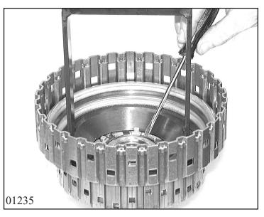
Press down cup spring B in the mandrel press with assembly bracket 5x46 002 566 and take out the snap ring. Remove washer and cup spring.
