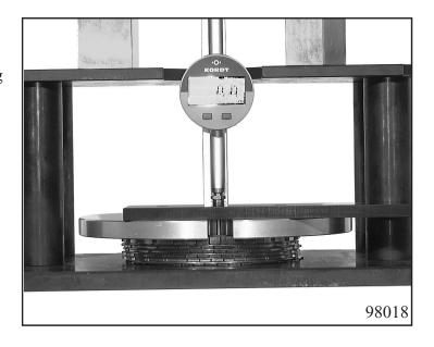
Now use the measuring bar to measure down to the base plate.
