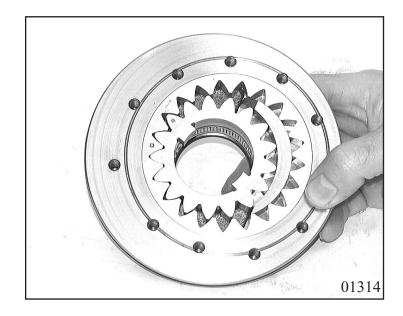
Pull 2 cylindrical rings 10.040/160 + /170 onto the stator shaft 10.040/120. So that the stator shaft can be mounted on the intermediate plate, these must be positioned towards each other. Follow the procedure stated on the next page.
