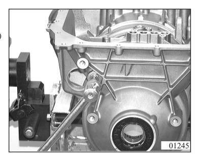
Press pin out of transmission casing. The ratchet with spring can then be taken off.
