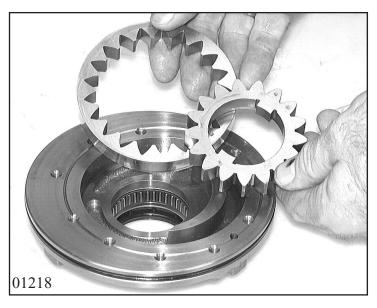
Pull off O-ring seal. The pump can be dismantled by taking out the impeller and ring gear.
